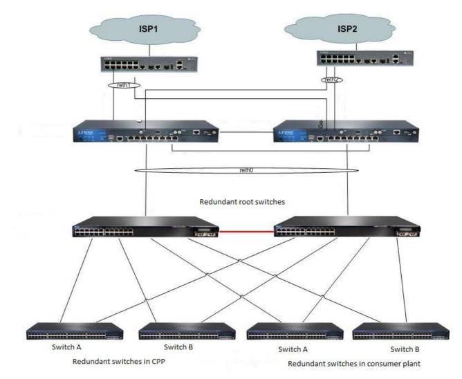
The above network diagram shows only the network switches for power plant and one consumer plant. By using the above shown network topology all process plants are connected in a single root switch. This enables the data communication between controllers of different plants.
