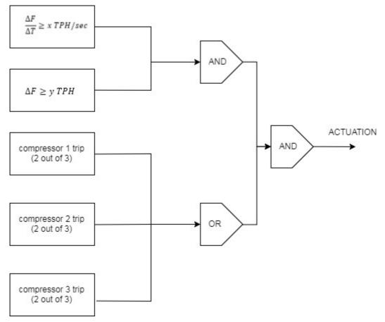
The actuation signal generated will manipulate the following parameters:
